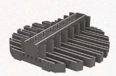
The liquid distributor LO is designed with troughs that feature lateral notches for discharge openings. These troughs are supplied by a parting box, enhancing the distributor's resistance to fouling and broadening its range of applications. The trough-type distributor includes a pre-distribution opening, known as a "parting box," positioned above several evenly spaced narrow troughs.
