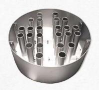
Pan-type distributors are devices used in packed columns to evenly distribute liquids across packing material, ensuring optimal contact with gas phases. Their flat, pan-like design features multiple outlets for uniform liquid flow, enhancing mass transfer efficiency and overall process performance.
